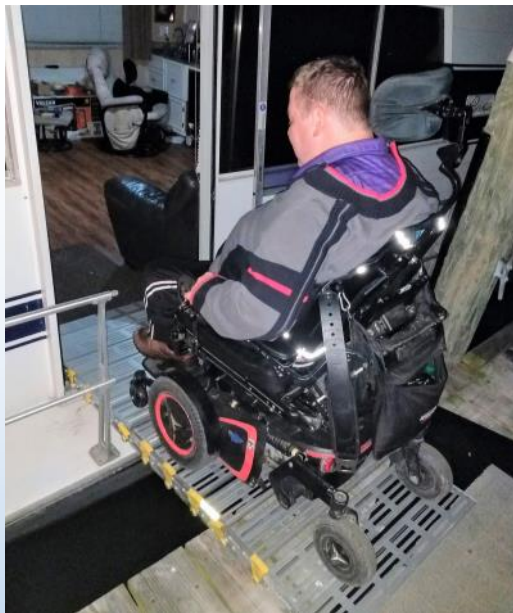
Pictured: 30" x 8' Boat Ramp, 1 handrail w/ Loop-End upgrade and secured with optional Seg-Mount Brackets
