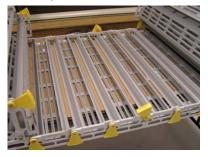
Step 6: Locate box wrench and allen wrench from your Owners Manual packet. Use these tools to tighten the connection on the ramp. Do not over-tighten. Position the caution cover over the pinch point on the side of the ramp.
